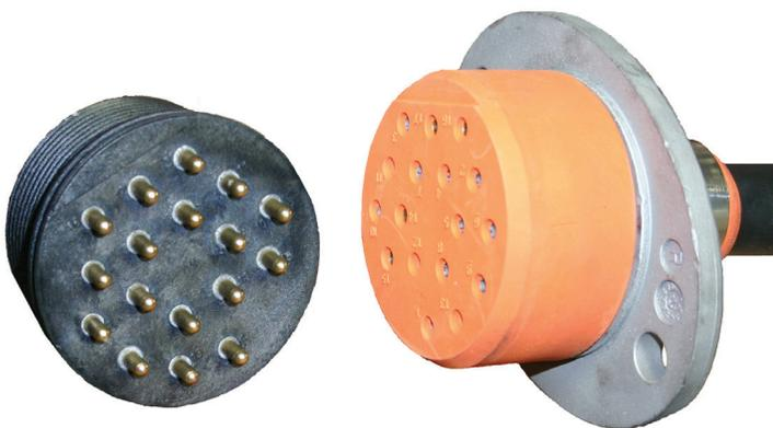
*For dual-voltage motors, an orange plug easily connects 460 or 575 volt power to male pins sealed into the top of the motor housing. A black plug provides 208-230 volt power without re-wiring the motor.*
