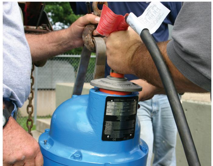
*When the stainless steel plate is bolted metal-to-metal against the motor housing, the connection is sealed to over 65 ft of submergence and is FM qualified for flame path resistance.*
